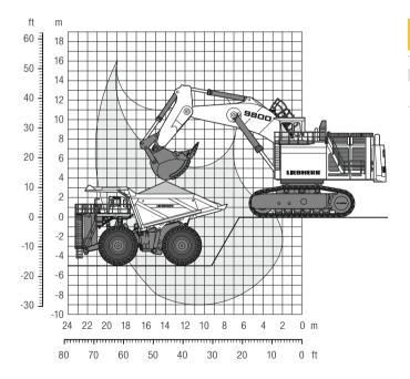
T 284 Mining Truck loaded by the Liebherr R 9800 hydraulic excavator in backhoe configuration
