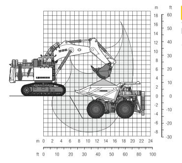
T 284 Mining Truck loaded by the Liebherr R 996 B hydraulic excavator in face shovel configuration
