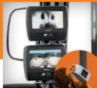
■ Four optional outside cameras can be mounted around the machine for enhanced visibility and help eliminate blind spots.
