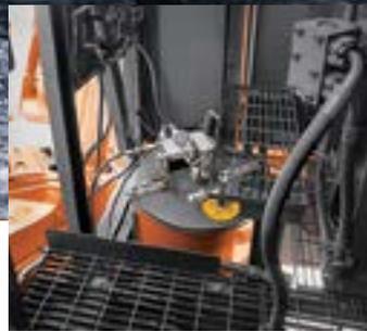
■ The compartment floor slides down to lower a grease drum can for quick replacement.
