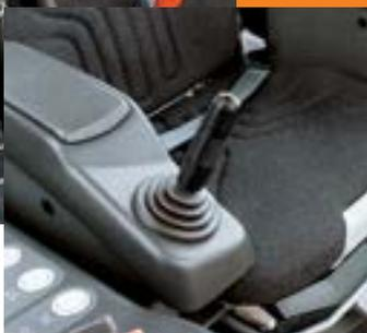
■ Electric joystick control levers provide precise and almost effortless operation.
