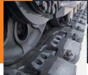
■ Rugged track links include roller guides to help extend service life.
