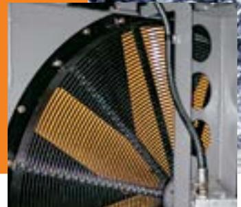
■ The oil cooler is strategically positioned far from the engine radiator for even better cooling potential.
