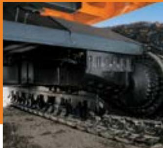
■ High-mounted compact travel motors are protected from rock damage. Optional travel motor guards provide an even higher level of protection from damage.
