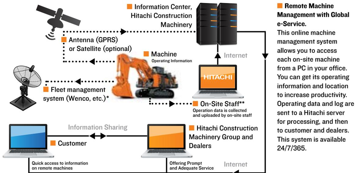
Note: In some regions, the Satellite Communication Device is not available by local regulations; the GPRS (mobile) communication device is an option for these regions.
