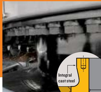
■ The cast steel structures, integrated into the center track frame, assist in avoiding stress concentration and increase reliability.
